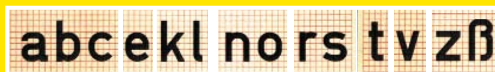
DIN 1451 'Mittelschrift' for hand lettering, preliminary version from 1931
