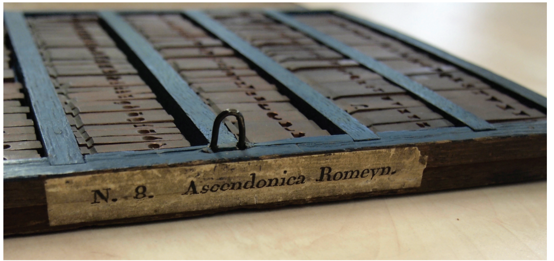
Set of matrices (MA8) of Granjon's Double Pica Roman or Gros-parangon (1570).
